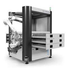
Up to four gripper change systems can be integrated in the X-CELL WB. This means that multiple orders can be processed automatically without the operator having to change the gripper. An integrated reversible gripper enables machining of the sixth side without manual reclamping. The single, double, and special grippers are all equipped with an integrated blowing nozzle and position monitoring for component recognition.
